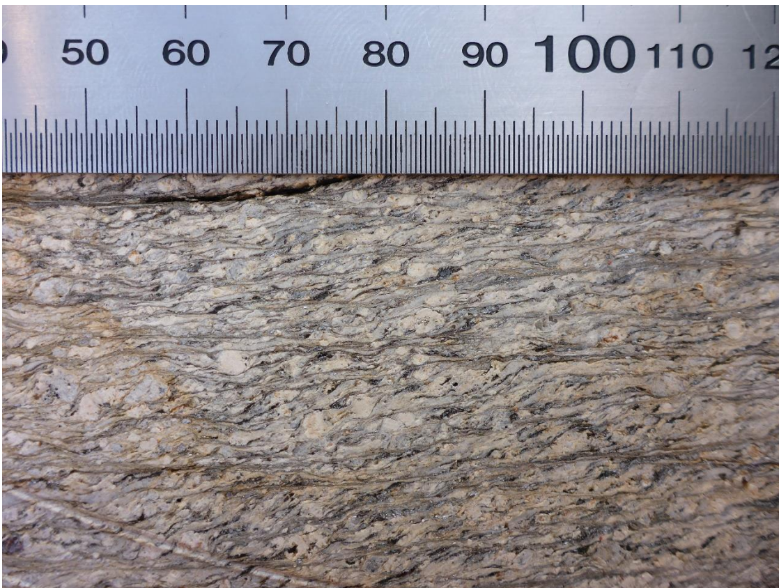
Figure 2 Cut surface oriented perpendicular to foliation and parallel to lineation. Top-to-the-right shear sense indicated by S–C fabrics in this view translates to sinistral strike-slip shear sense at the outcrop. Major increments of scale are 10 mm.
